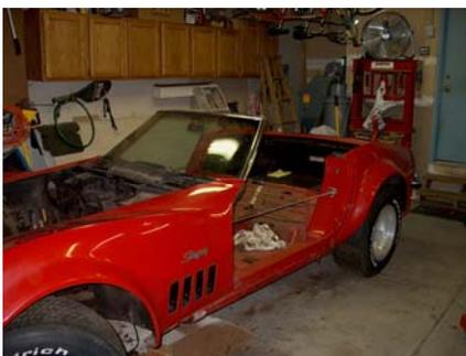
and all other misc exterior trip and chrome. He had also put stabilizer rods in the door posts to keep the body from flexing. Prior to starting, Pete had removed all the body mounting bolts, so all that remained was the easy stuff!
