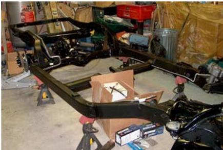
Such is not the case. The frame is finished however after sand-blasting, cleaning and being treated with a fresh coat of paint, it looks as good or better than the day it ran down the assembly line in St Louis.
